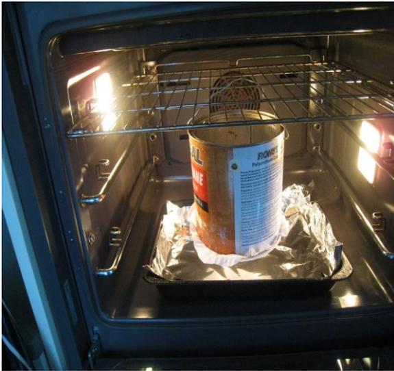
**Oven fitted up, ready to melt and filter wax**
