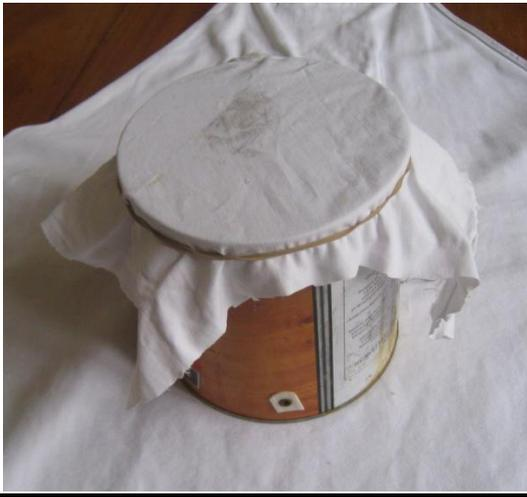
**Filter being attached to the tin**
